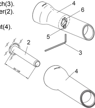
**NOTE:** Do not overtighten the setscrew.
