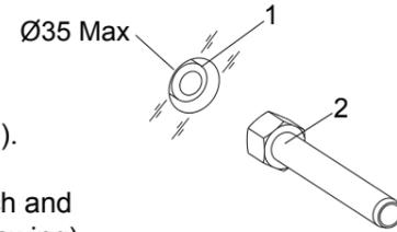
2.) Apply tape or thread sealant to G1/2" threads of the male supply fitting(1).
